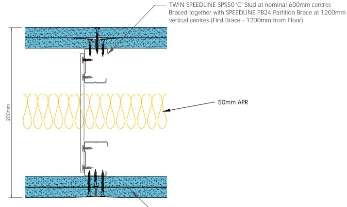
2 layers of 15mm Siniat GTEC dB Board fixed with SPEEDLINE Drywall Screws at 300mm centres (200mm centres at external angles). Ref to table for fixing length.
